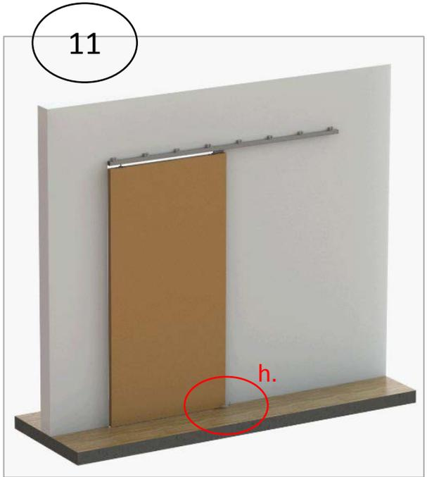
Place guide on the floor halfway in (h2.), secure with screw (h3.)
