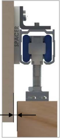
Slide brackets onto track and fix them with screw supplied (c1. and c2.). With track in a levelled position and secure with screws (c3. and c4.).
